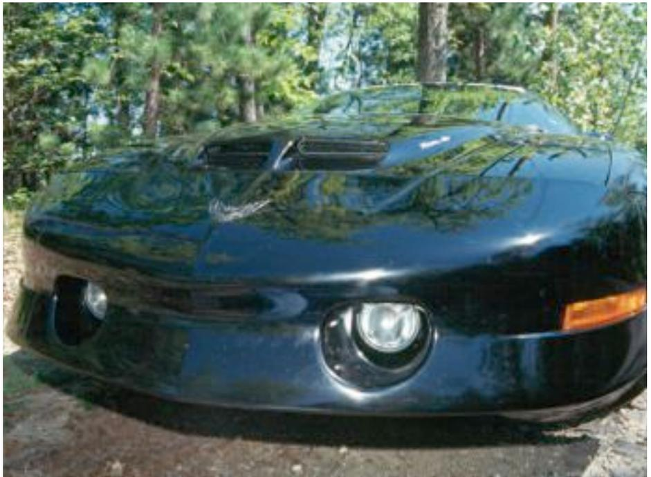
**A composite Ram Air hood was also added to give the supercharged V-6 cool air to breathe. Engine was incredibly responsive and free-revving.**
