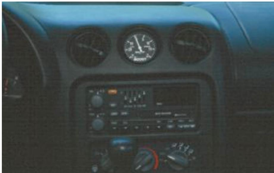
**The interior of the Trans Am was left 100% stock, except for a single boost gauge that was put in the center air vent located in the dash. Boost was limited to 8.4 psi.**
