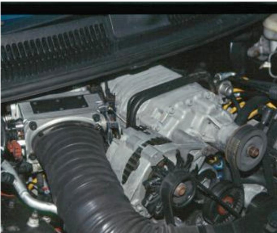
Closeup of induction system shows the LT1 throttle body and the Holden V-6 inlet elbow. Blower drive precludes a front TB inlet- air must enter at the rear.
