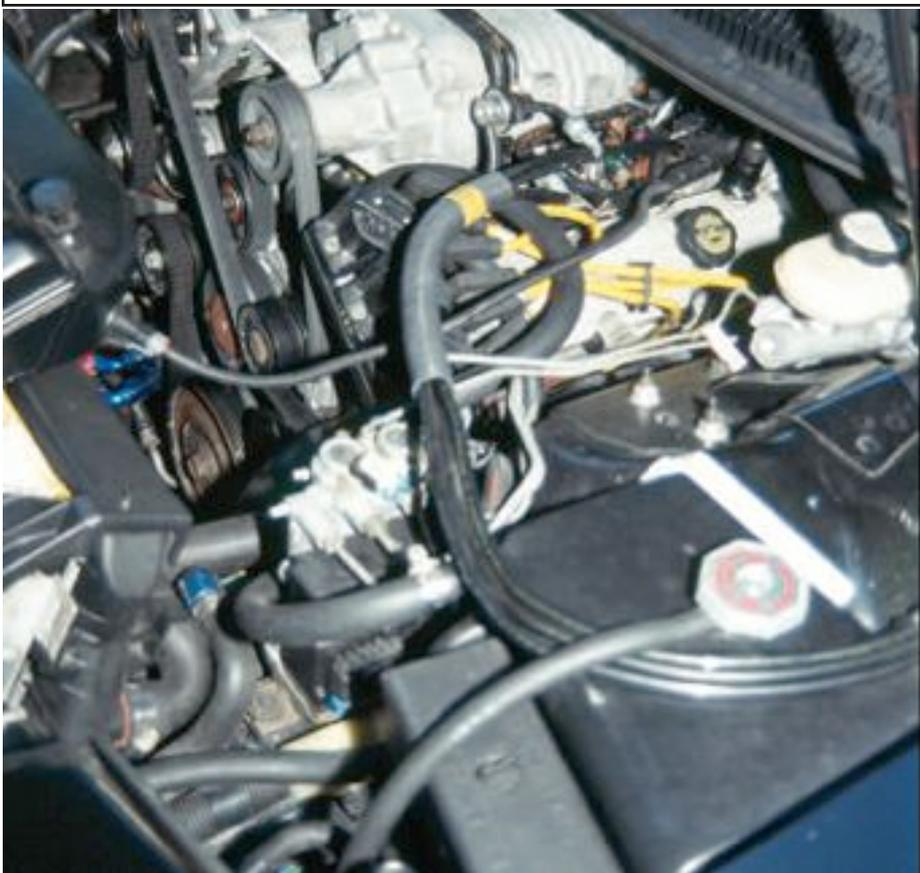
The reservoir for the air-to-liquid intercooler was located on the driver's side of the engine compartment. The system used a mild glycol solution.
