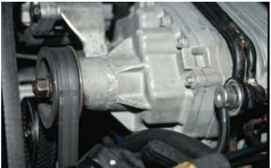
**The Eaton Model 90 drive snout was lengthened to line up with custom accessory drive.**
