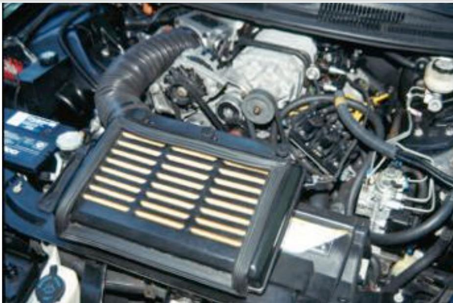
Though there was ample room to fit the supercharged V-6, it still looked pretty busy in there. Custom air cleaner looked similar to stock WS6 unit but air was routed to the passenger side rather than directly back. It used the stock WS6 filter element.
