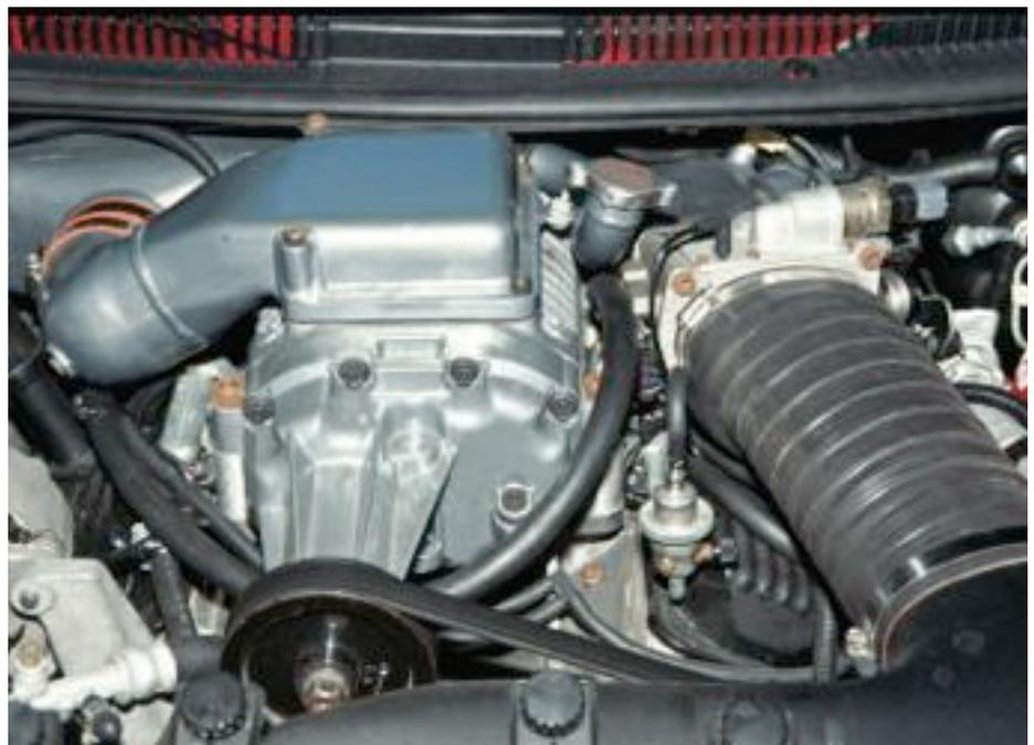
The supercharger was a prototype 112 cubic-inch Eaton unit similar in design to the 90 cubic-inch version used on the Grand Prix GTP's L67 V-6. The larger pulley kept the boost to about 8.5 psi, though more boost and power was available if needed with a smaller-diameter pulley.
