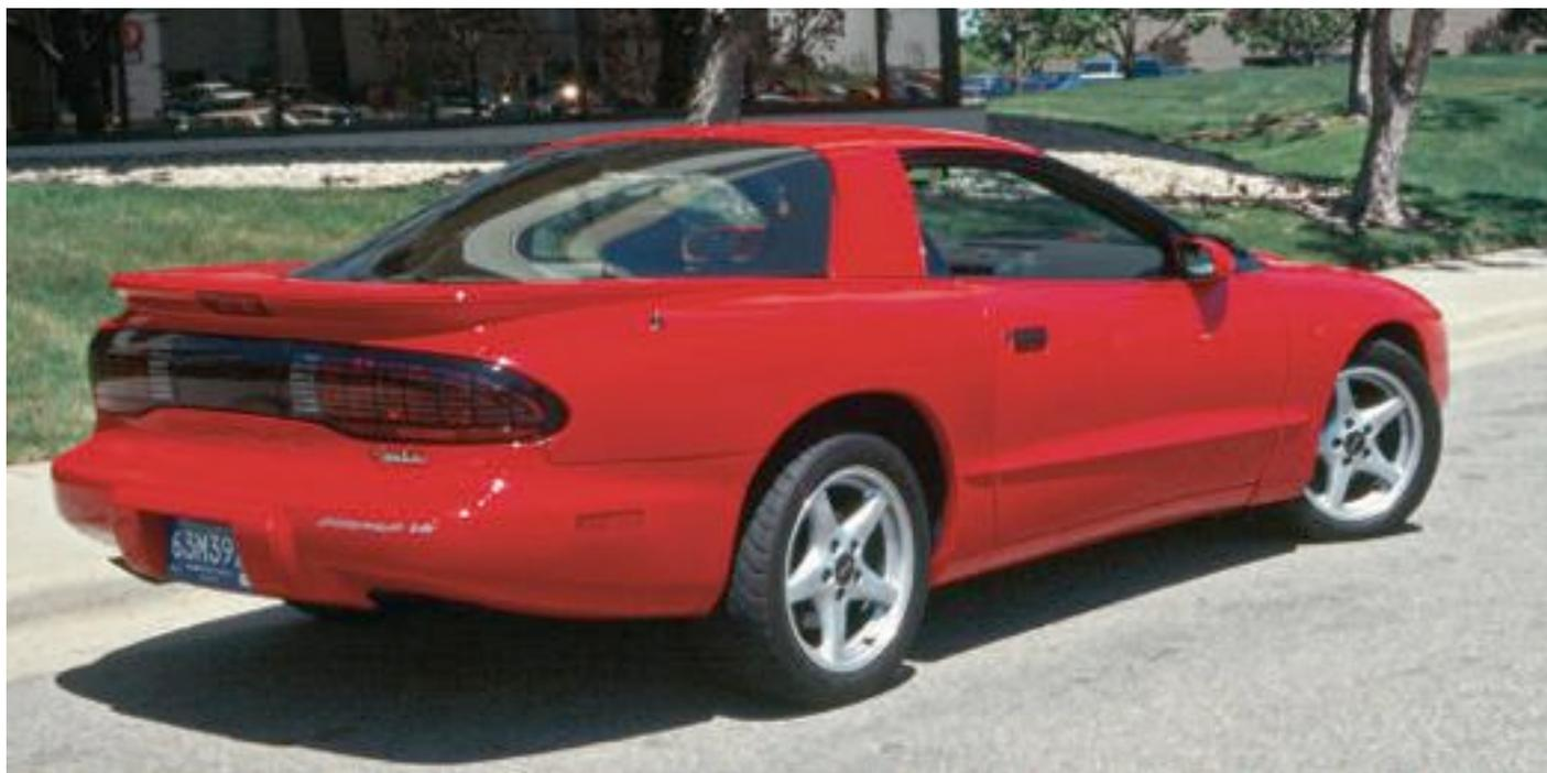
Though tough to see, the rear-bumper fascia for the stock Formula has an empty spot where the passenger-side exhaust pipe would have gone. This car received a prototype version of the high-flow, single-outlet system that made it to production on the '98 WS6 Firebirds.
