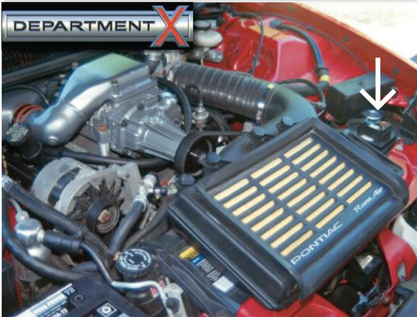
A tank for the air-to-liquid intercooler was mounted near the radiator-core support (arrow). It held a mild glycol solution that was pumped into the cooling element in the blower manifold to reduce charge-air temperatures.
