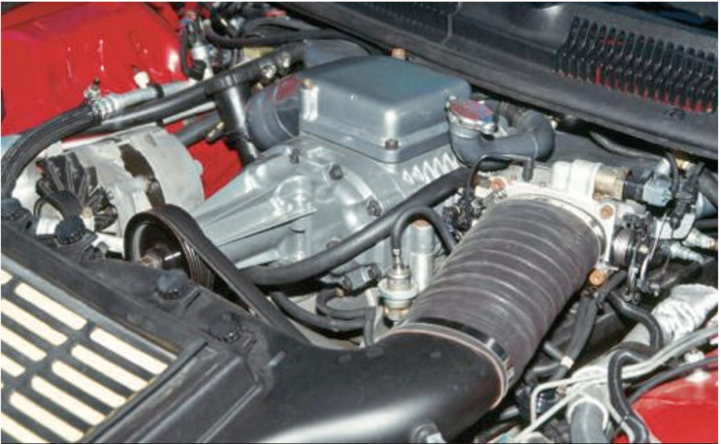
With the conventional top-entrance of the blower design, the air was routed into the throttle body and then behind the blower and around the other side. All of the ductwork to accomplish that task was custom fabricated. An air-to-liquid intercooler sat just under the supercharger.
