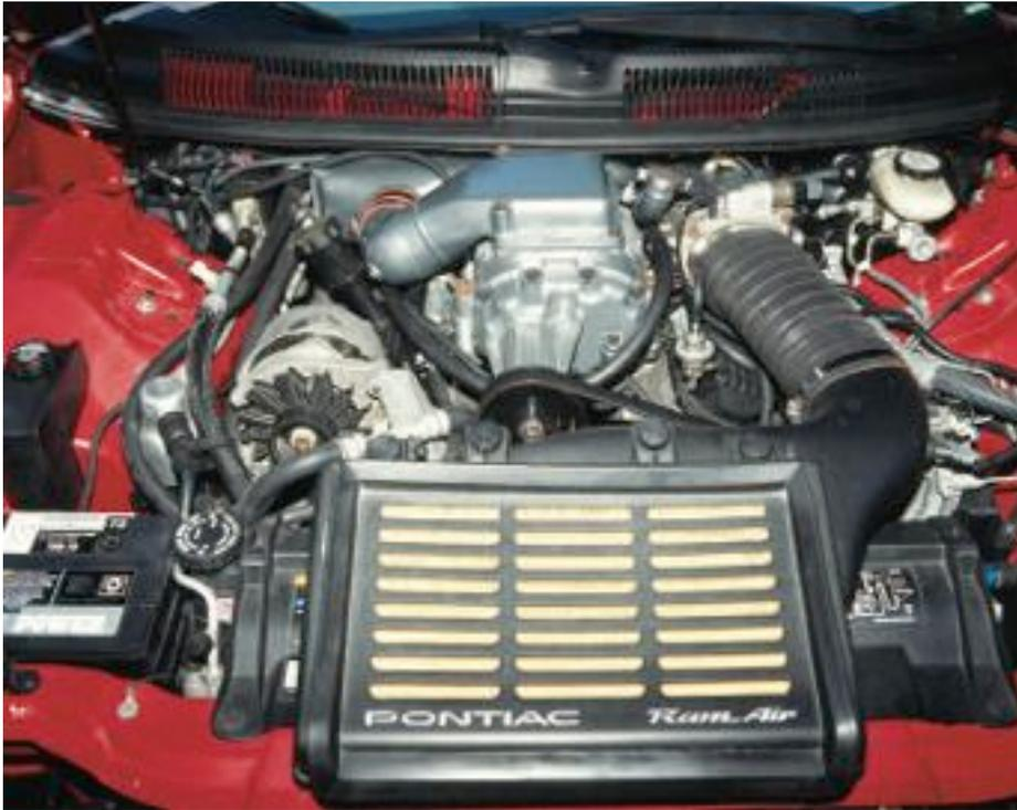
**The Ram Air system used a production hood with a non-production airbox that routed air to the driver's side of the engine compartment. This housing used a stock WS6 air filter. Plastic ducting routed air to the LT1 throttle body.**
