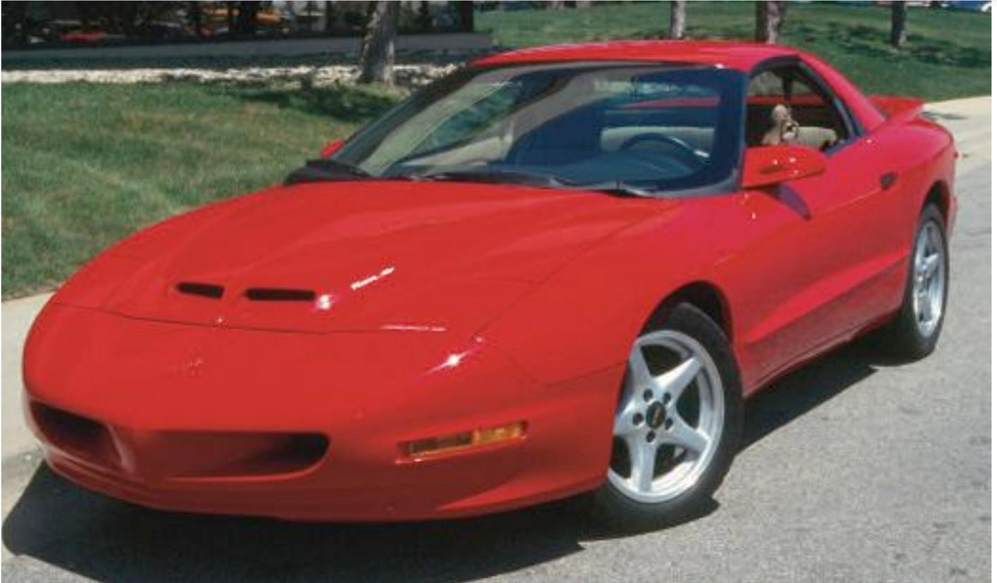
Pontiac Special Vehicle Engineering built this Firebird Formula with a supercharged 4.3L L99 V-8 engine to test the performance potential of a smaller-displacement engine in a Firebird application. The steel-roofed Formula was an early '93 model, upgraded to WS6 specs.
