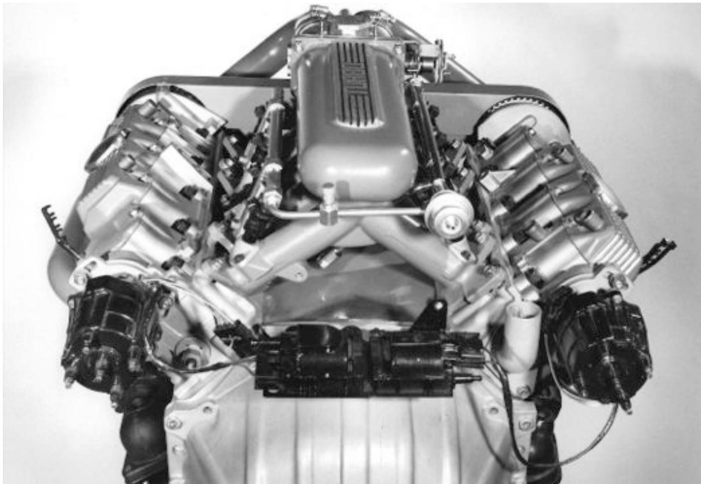
Custom-fabricated intake manifold housed specific throttle body and stock Sunbird Turbo injectors.
