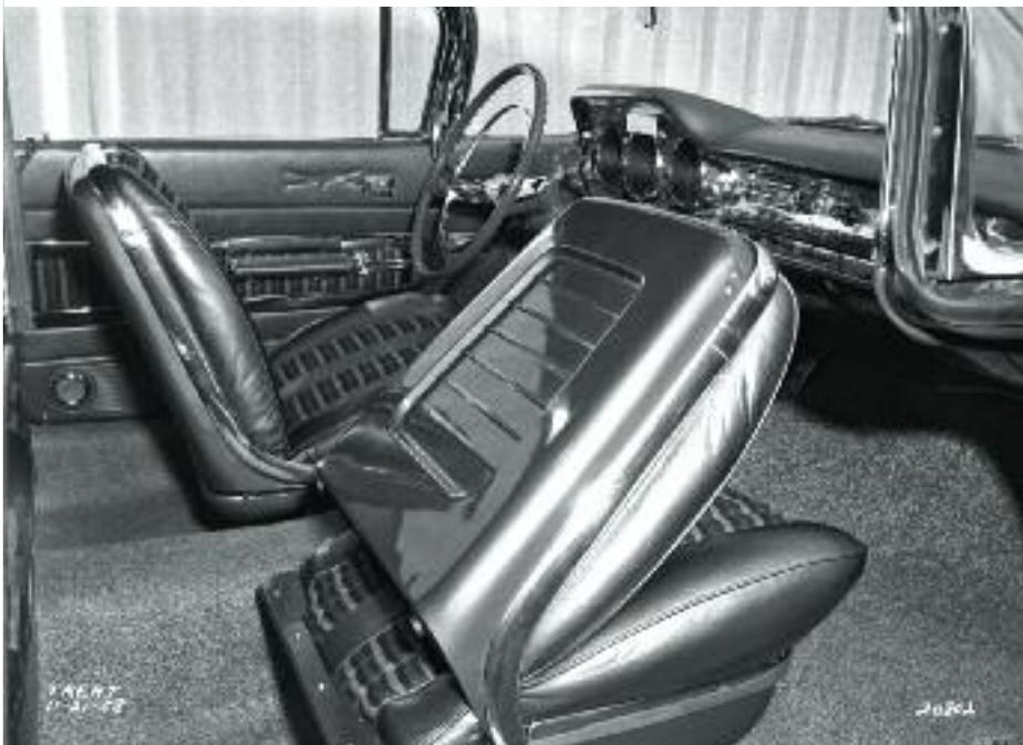
This shot of the 1959 Ventura Custom Coupe was taken on November 21, 1958, and shows the blend of production and non-production elements used. The hard-shell bucket seats featured cloth and Morrokide upholstery, the former appearing to be a pattern similar to what was used on 1959 Chevy Impalas. Note the power wing window controls, a detail that would not reach production until 1963.
