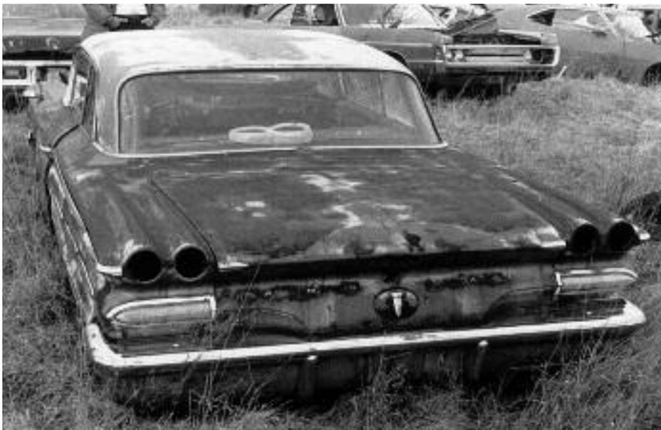
**At the time that the car was photographed in 1988, all of the non-production glass was still intact. The car was known to local Pontiac fans as the "fiberglass roof car." The item on the rear deck was a non-production plastic headlamp bezel, the same type as used on the 1960 X-400.**
