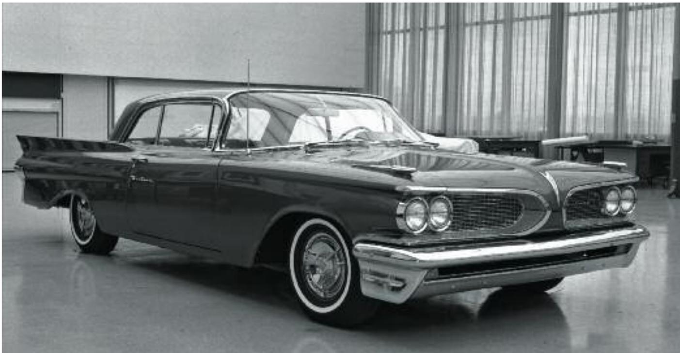
The 1959 Ventura prototype clearly shows that the basic elements of the Grand Prix had been established. In addition to the use of the shorter Catalina platform, this concept car features a formal roofline, an absence of side chrome and a tastefully restrained overall appearance. The soft bulbous designs and the abundance of chrome were being abandoned in favor of sharper, crisper lines and less trim. Clearly, a new generation of design was taking hold.
