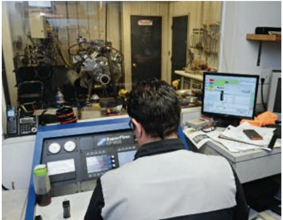
The 535 delivered on its promise for 700 streetable horsepower with a maximum of 701.1 horsepower at 5,800 rpm, with 718.6 lb-ft of torque at 4,900. This should not only wow the troops with its beautiful appearance, it will also be a torrid street performer when installed in the 2,500-pound '31 Pontiac coupe.
