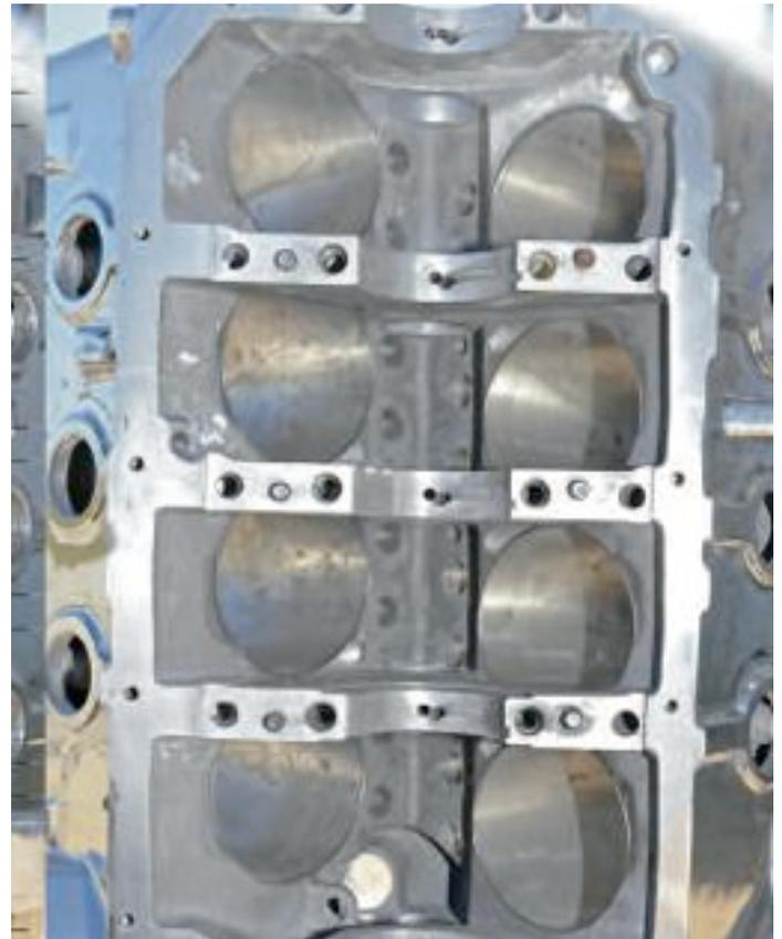
The aluminum IA2 is a beefy block and will be more than strong enough for twice the horsepower that this engine will be making. The 3-inch mains will support an Eagle 4340 4.5-inch, stroke forged-steel crank. Like much of the engine, it is overbuilt in case the owner is interested in turning up the wick with a hotter cam and head porting.
