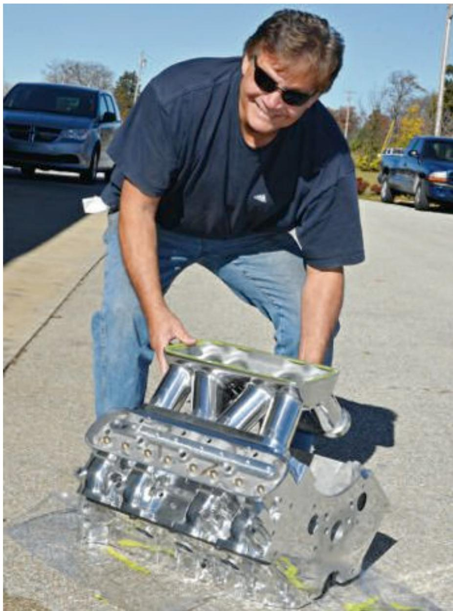
Lynn McCarty of McCarty Racing shows off the polished aluminum pieces that will go into the build of this all-aluminum 535 cubic-inch Ram Air V. AllPontiac.com block is topped with McCarty Racing reproduction tunnel port heads and matching tunnel ram intake manifold. The polishing was handled by P&C Metal Polishing in Cincinnati, Ohio. This engine will be installed in a 1931 Pontiac street rod. Even in a mild state of tune, this will be a delightful dose of overkill.
