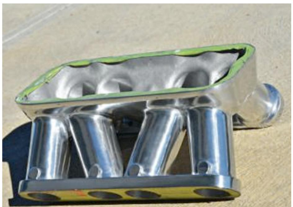
The tunnel-ram intake is designed to accept a variety of tops and has injector bung pads cast in for use with both carbureted and EFI induction systems. There is also plenty of material cast-in for porting. This particular build will have it mounting a pair of Holley carbs.
