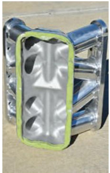
The inner contours of the McCarty tunnel ram show the smooth, well thought-out design. A variety of tops are available for single or dual four-barrels or Holley-based throttle bodies. A custom top for an EFI throttle body could also be fabricated and used, depending on the design requirements, making this intake a great choice for forced-induction applications.
