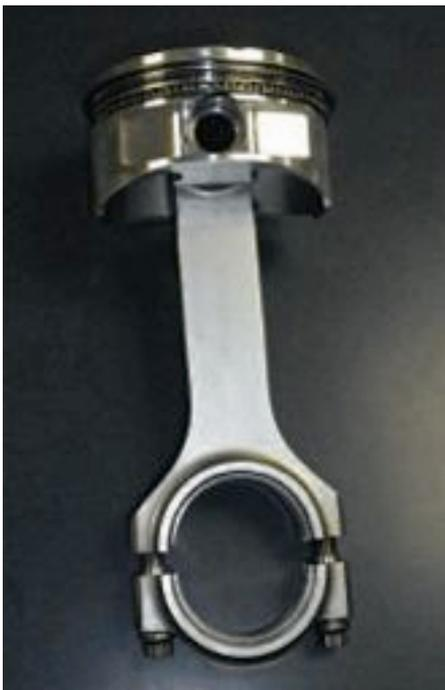
The piston and rod combination is the tried and true Ross forging with a 4.35-inch bore size and Eagle 6.8-inch 4340 forged steel rods. This build required a 20 cc dish in the piston to keep compression at 10.5:1.
