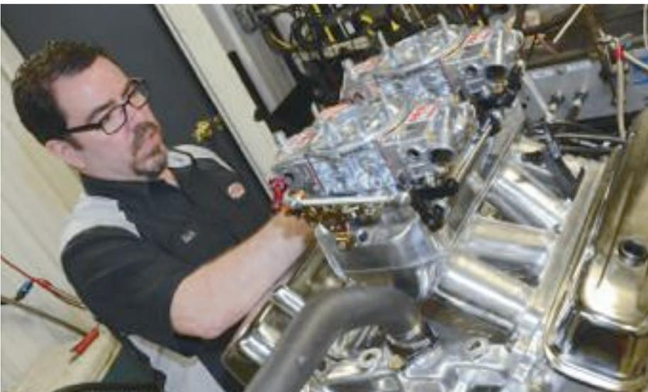
Running two 850-cfm carbs on any size street engine is going to make for sluggish performance but Lynn thought ahead. The sideways-mounted carbs feature a progressive Enderle linkage kit, which only opens the front barrels of each carb under part-throttle operation, dramatically improving driveability. Here, Rich adjusts the linkage in preparation for a dyno pull.
